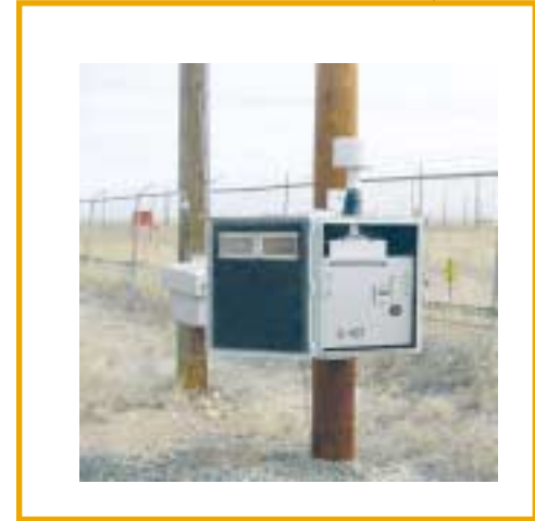
Data collected from air-monitoring stations like this one, near the 903 Pad, are used to quantify actinide movement by the wind. Air is a major transport pathway.
