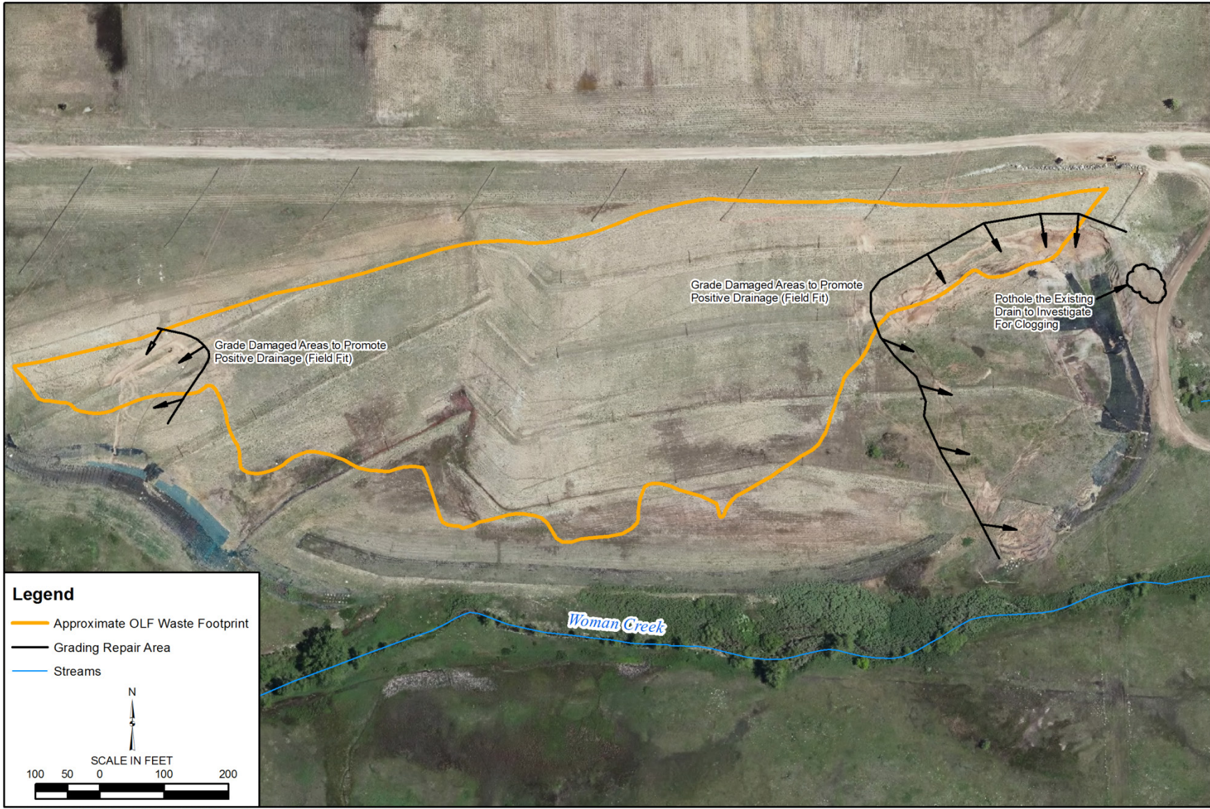
Figure 2. Original Landfill Interim Repairs Sketch Layout—September 2015
