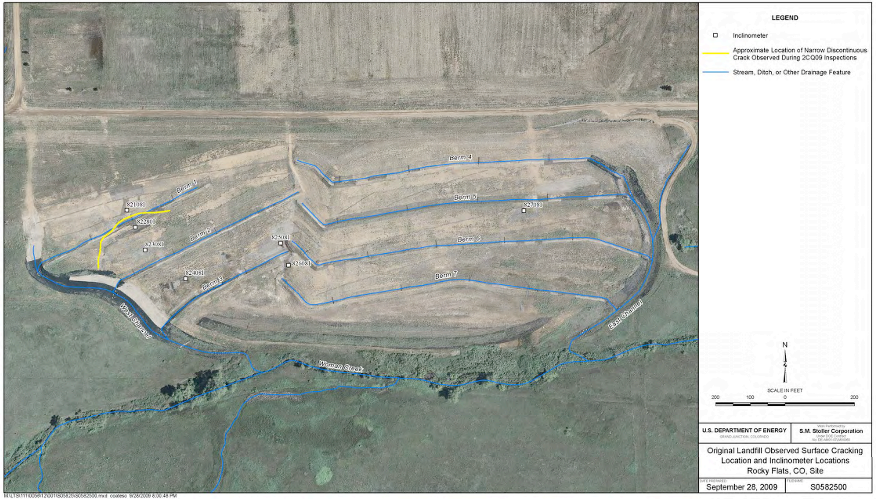
Figure 1. Original Landfill Observed Surface Cracking Location and Inclinometer Locations
