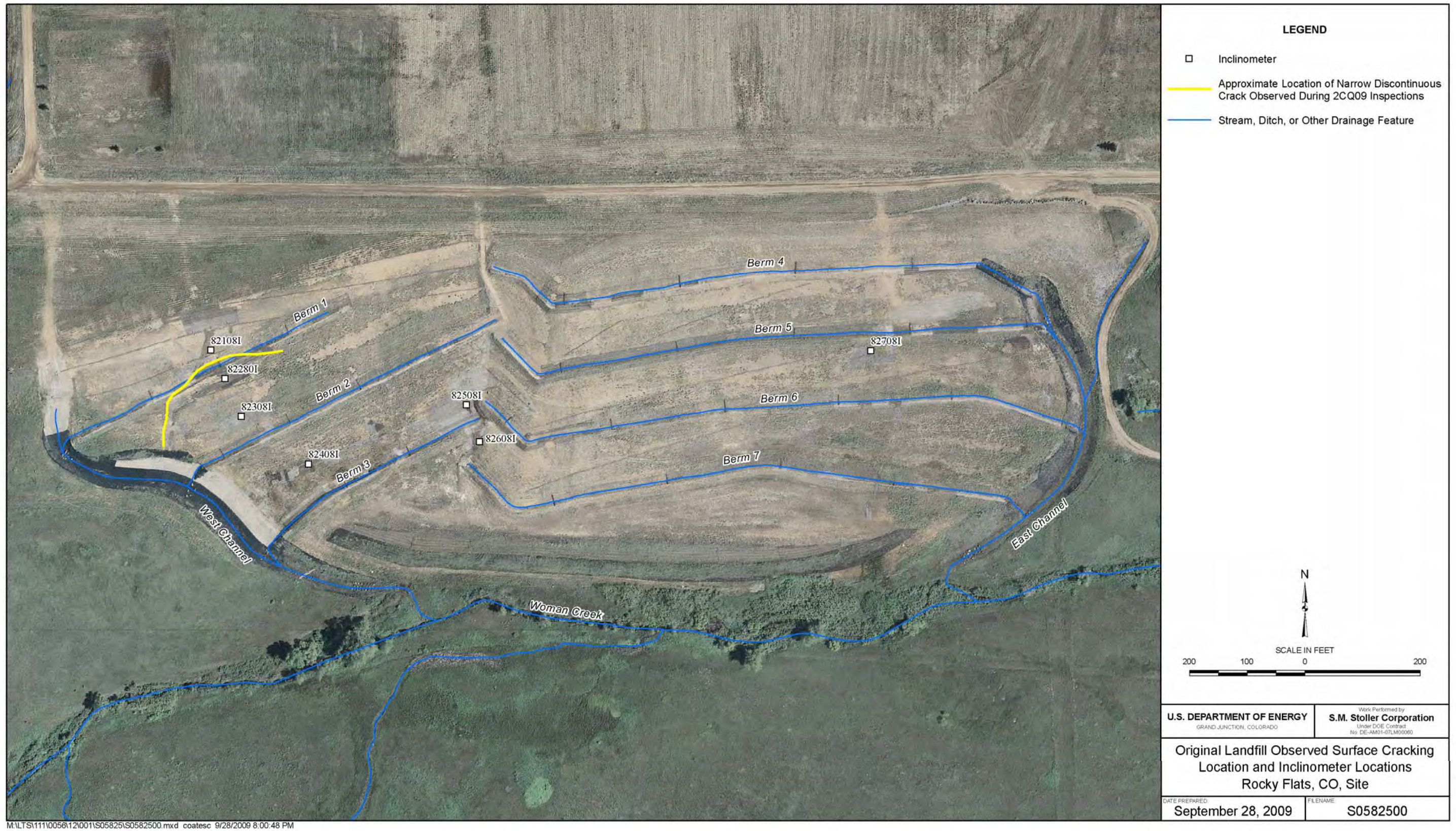
Figure 2. Original Landfill Observed Surface Cracking Location and Inclinometer Locations
