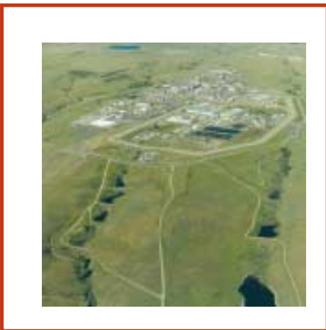
The actively managed detention ponds on South Walnut Creek (left) and North Walnut Creek (right) settle out 80 to 90 percent of the plutonium and americium loads carried into them from runoff.
